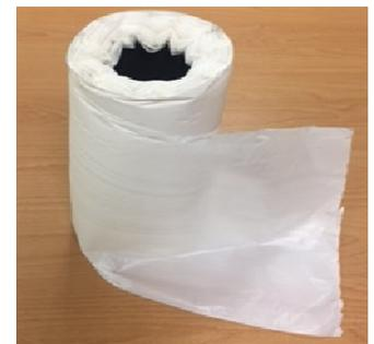
Picture 1: Compound BIO563 is easily processed in conventional blown film extrusion lines
