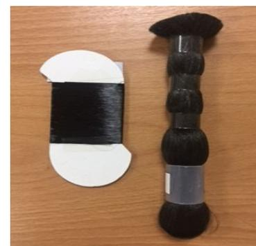
Picture 3: Black PT6302 is a proven solution for the coloration of polyester fibers.
