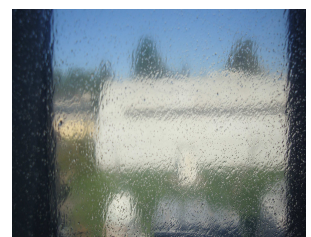
Picture 3: The new masterbatch 001 П0АБ25 creates visible antiblocking spots on the polyethylene film.
