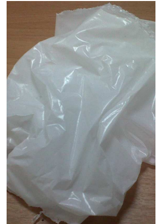
Picture 2: Filler 5706 can be loaded up to 30% in a breathable film formulation.
